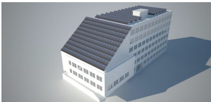
Fig. 7. Proposal of photovoltaic system
