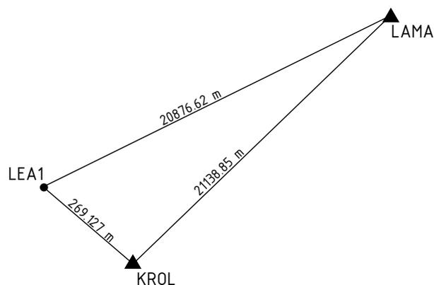
Fig. 8. Draft of adjusted vectors
