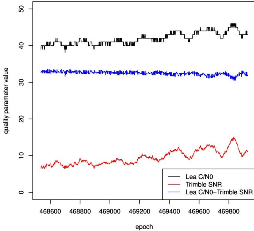
Fig. 2. Difference in C/N0 and SNR value
