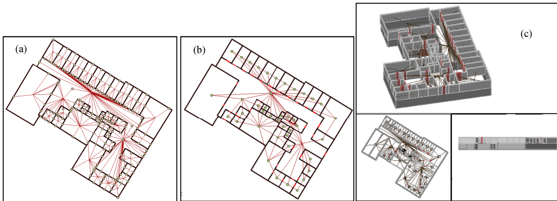
Fig. 4. Network models developed with the use of CAD tools based on transformed data sets; a) model C_{xyh}^{LR} , b) model C_{xyh}^{LKR} , c) visualization of two floors in a building
