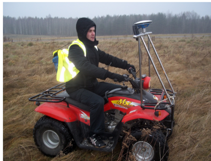
Fig. 2. ATV vehicle equipped with GNSS receivers and data teletransmission system. Self study based on GNSS tools
