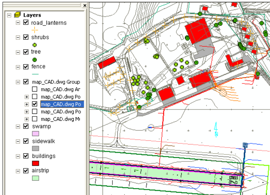
Fig. 1. Fragment of layers with vectorised linear and point objects on the background of the airport (EPOD) map
