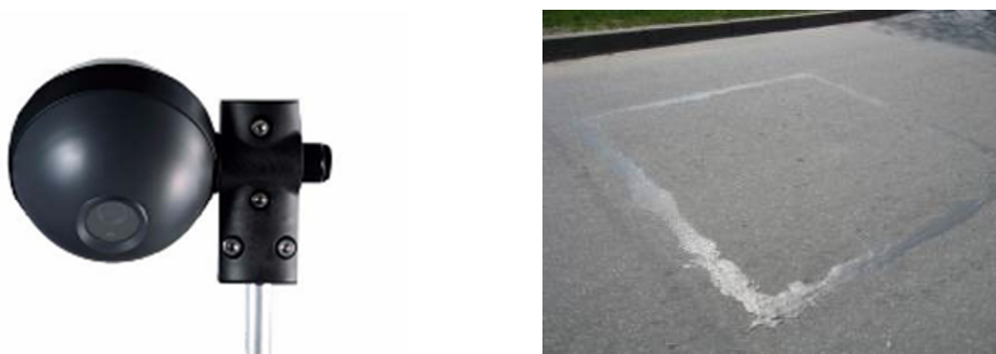
Fig. 3. Video detection in left side, induction loop in right side
