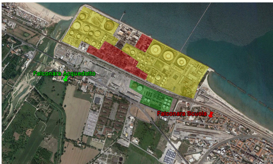
Fig. 4. Location of Falconara Scuola (FSS) and Falconara Acquedotto (FAS) monitoring stations and oil refinery; each area of the plant is branded by a color: the oil storage area is branded in yellow, the process area is branded in red, and the refined-product storage area is branded in green [7]
